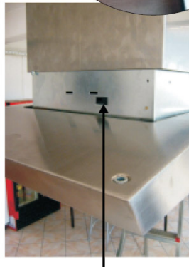
Hanging hook channel on motor cabin (Fig. 12b)
